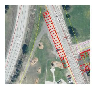
This first alternative consists of paving a single row of parking lot, providing approximately 20 parking spaces plus 2 wheelchair accessible spaces.
